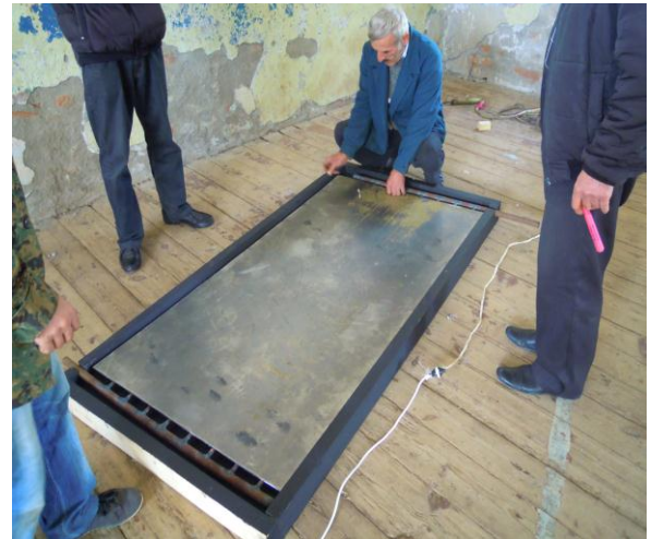
Photo by: RCDA Constructing solar water heater
